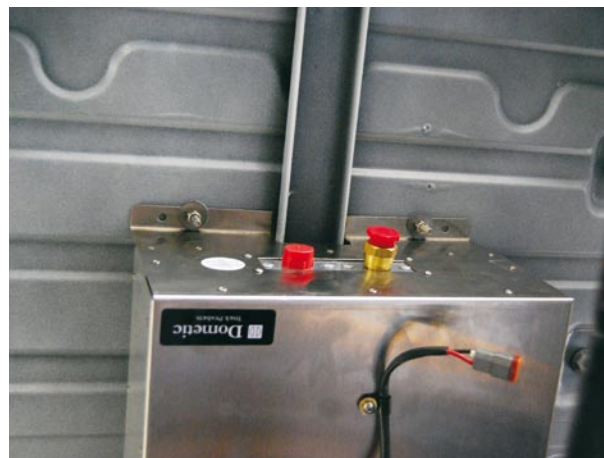
Figure 2b - Condensing unit mounted under truck
